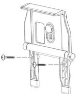
2. Connect the USB cable and secure the clip knob firmly to prevent it from falling off
