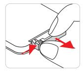
2. Install new battery into the compartment. Remove the old battery and install new one (CR2025). Ensure that the side with a "+" is facing up.
