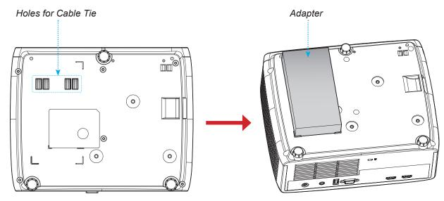
2. Secure the AC adapter with the cable tie.
