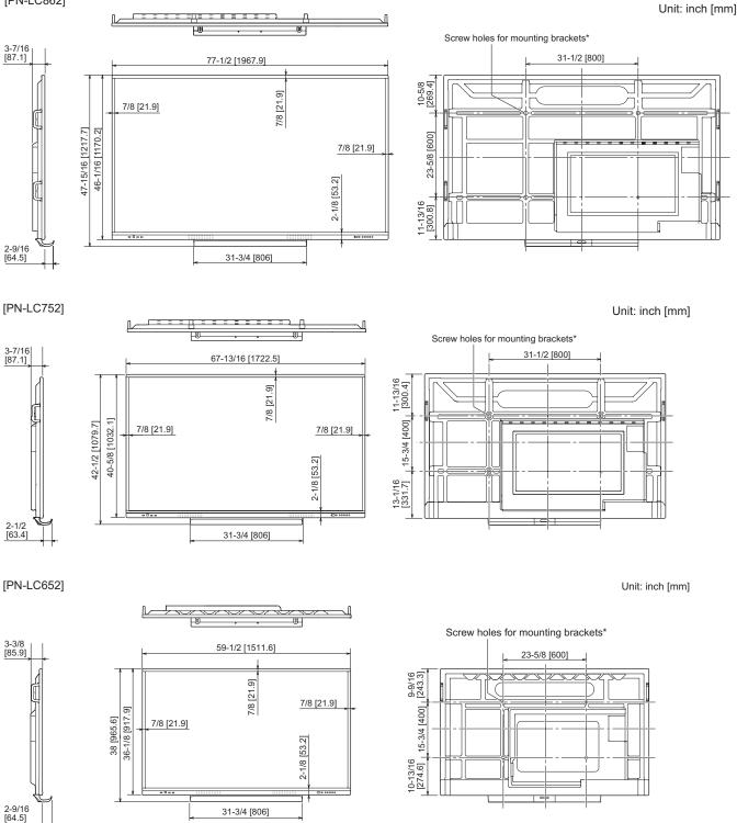
\* When mounting the monitor, be sure to use a wall-mount bracket that complies with the VESA-compatible mounting method. SHARP recommends using M8 screws and tighten the screws.
