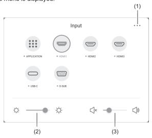
Press the  $\blacktriangle \nabla \blacktriangleleft$  or  $\blacktriangleright$  button to select the input mode, and press the ENTER button to enter.
