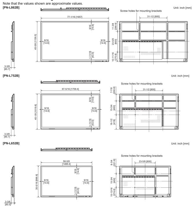
When mounting the monitor, be sure to use a wall-mount bracket that complies with the VESA-compatible mounting method. SHARP recommends using M8 screws and tighten the screws.
