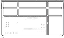
This monitor should be used at an ambient temperature between 41°F (5°C) and 95°F (35°C). Provide enough space around the monitor to prevent heat from accumulating inside.
