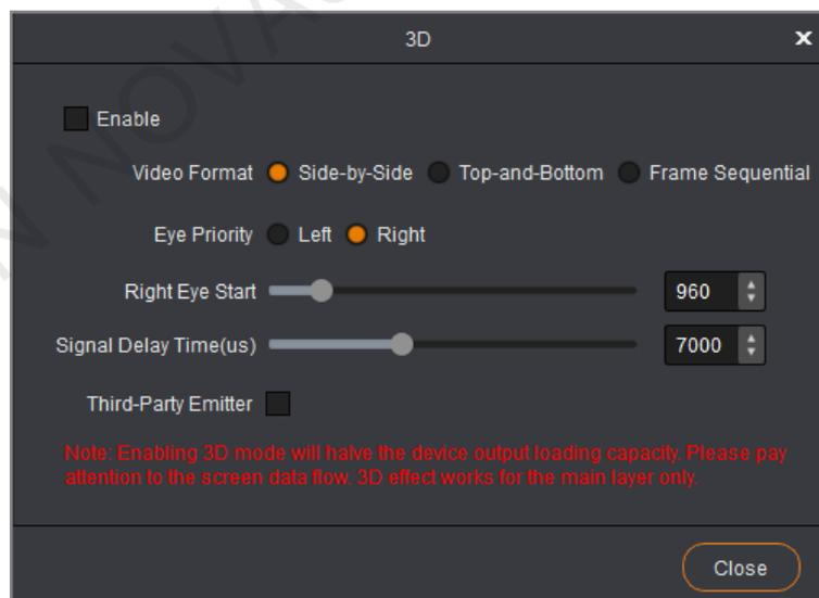
Step 3 Select the 3D format of the video source. The options include **Side-by-Side**, **Top-and-Bottom** and **Frame Sequential**.
