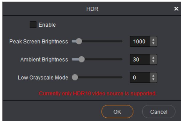
Step 2 Select **Enable** to turn on the HDR function.
