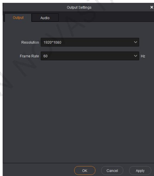
Step 2 Select a desired output resolution for the HDMI connector from the drop-down list next to **Resolution**.
