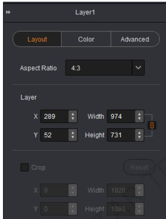
Step 3 Set the aspect ratio, size and position of the layer according to your actual needs.
