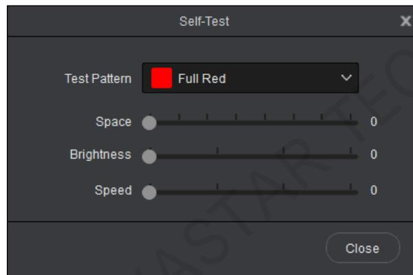
Step 2 Select a desired test pattern from the drop-down list next to **Test Pattern**.
