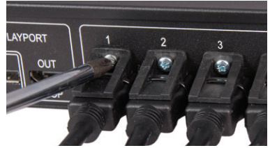
Connecting HDMI Output Cable
