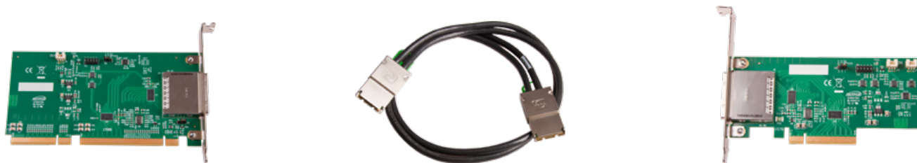
Fig2: PCI Express Link containing HLink-G3, ExCable-G3 and SLink-G3
