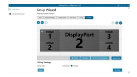
If you chose to have the DDCT configure your wiring, this page will display the recommended display connections, as shown above. Connect each display to the corresponding output connector on the rear of the VSN wall controller. The printed input/output diagram shipped with the your VSN wall controller shows where the display connectors are located on your system. If your VSN wall controller is connected to a printer, you can print a copy of the wiring diagram using Print a Wiring Diagram.
