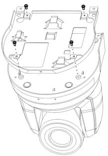
3. Lock the metal plate B on ceiling mounted hanger
