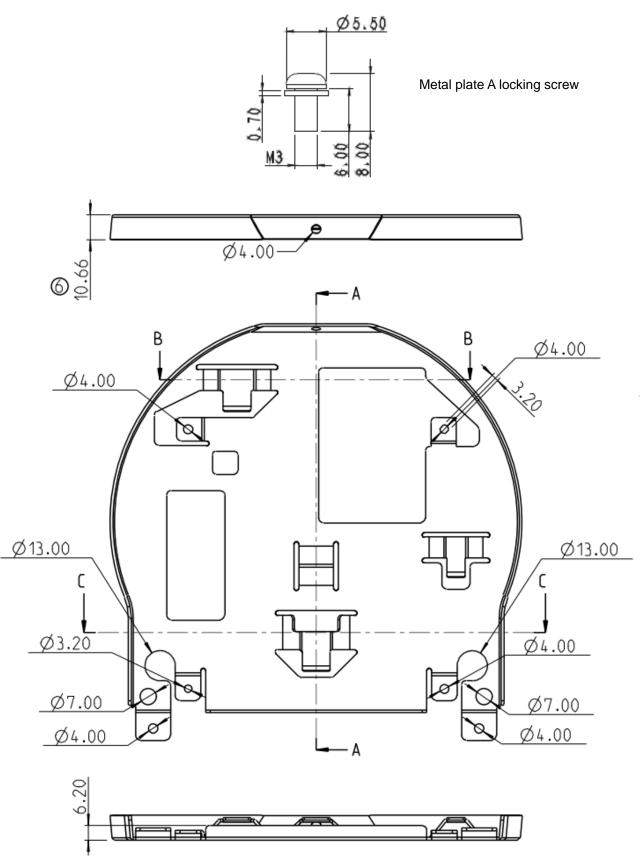
Metal plate A - machine side
