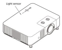
Do not block the light sensor when using automatic image quality correction based on the ambient brightness.
