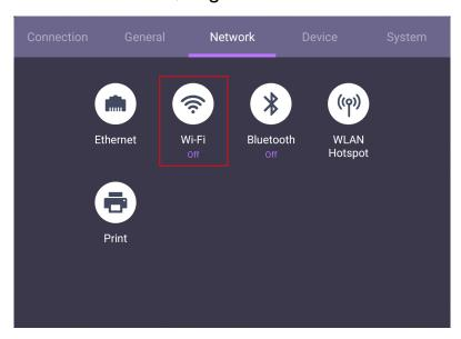
2. Insert the Wi-Fi dongle and the switcher will automatically change to **ON**. A list of available networks will show on the screen.
