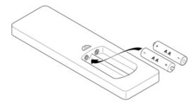
3. Replace back cover on the remote control and press down until it clicks in to place.
