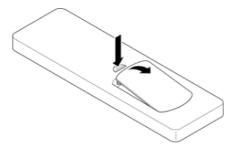
2. Insert AAA batteries in the battery compartment. Ensure each battery's polarity (+/-) is aligned correctly.
