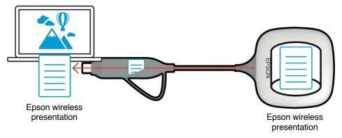
(b) Epson wireless presentation (software) converts content on your computer (Windows/Mac) into the transmittable data and transmits the data from the transmitter to the receiver over a wireless LAN (Wi-Fi).
