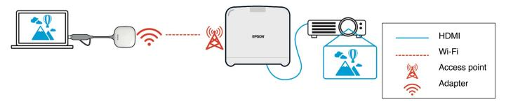
(b) Wireless LAN (Wi-Fi) connection between a computer with Epson iProjection installed and the receiver
