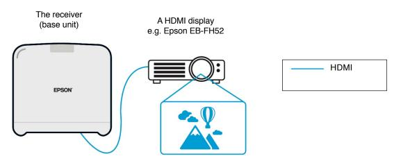
If the display is a supported Epson projector, the function of the receiver (base unit) can be built into it. The base unit model and supported Epson projector model receivers have the same function, to receive transmitted data over the network. The base unit model and the supported Epson projector model are both described as 'receivers' unless otherwise noted. Illustrations used show the base unit model receiver.
