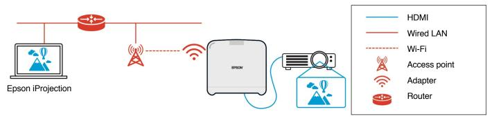
(b) Wired LAN connection between the receiver and the infrastructure network
