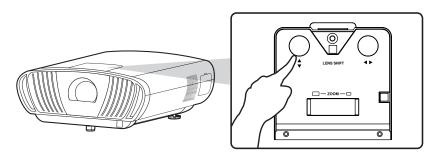
**CAUTION:** Do not rotate the lens shift knob any further when you hear the click sound. Overturning the knob may cause damage. Press down on the lens shift knob to rotate back.
