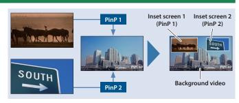
5. Use the PinP 1 [POSITION H] and [POSITION V] knobs to adjust the display position of the inset screen.
