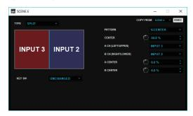
When you move the cursor to the screen split display area, the mouse pointer changes shape. You can use the following mouse operations to adjust the display position of the video and the split position of the screen.
