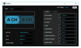
When you move the cursor to screen A or screen B, the mouse pointer changes shape. You can use the following mouse operations to adjust the position and size of the screen.
