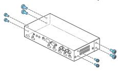
Using the screws that you removed, attach the rackmount angles as shown in the illustration.
