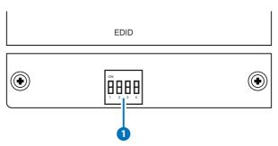
1 EDID: EDID switch offers EDID selection. There are 16 sets of EDID selection totally which divide to three modes includes "internal mode", "user mode" and "native mode". 6 set of internal EDID, 9 sets are defined as user mode which are allowing customer to upload as prefer one. The last one is native EDID which copies EDID from sink device.
