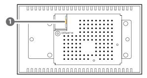
**1 CAT5e/6/7 IN:** Connect to the transmitter unit with a single CAT5e/6/7 cable for transmission of all data signals and power.
