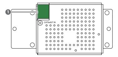
**CAT5e/6/7 IN:** Connect to the Transmitter unit with CAT5e/6/7 cable for transmission of all data signals.
