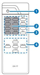
3 ALL: Press this key to select all outputs simultaneously for routing. Next, press the key of the input (1~4) you wish to route to all outputs. Finally, press "ENTER" to confirm your selection and execute the routing change.
