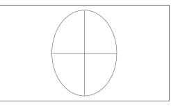
An anamorphic lens will stretch the image horizontally, restoring the original 2.35 ratio:
