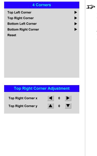
**Corner corrections provide a simple** setup for awkward installations and irregular shaped screens that may distort the image. To apply a similar (but less flexible) correction, while preserving the original aspect ratio of the image, use the **Keystone** menu.
