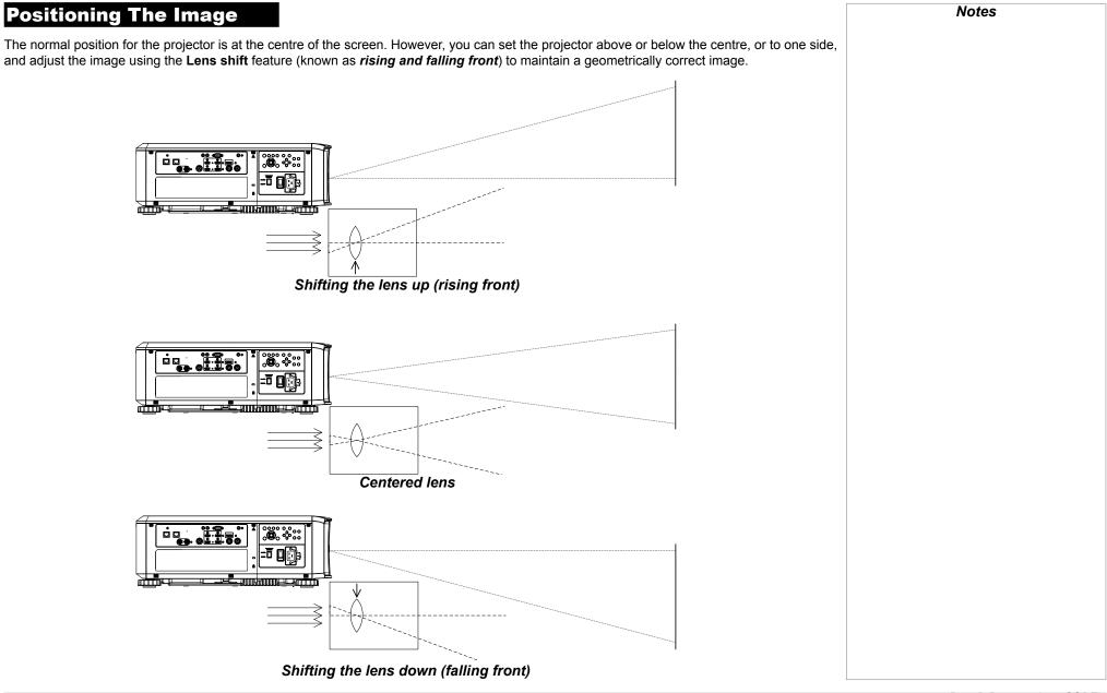
Any single adjustment outside the ranges specified on the following page may result in an unacceptable level of distortion, particularly at the corners of the image, due to the image passing through the periphery of the lens optics.
