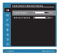
Press the **Menu/Exit** button on bottom right of your VSD243 to launch the OSD configuration screen. The OSD configuration screen can be used to configure the Contrast/Brightness, Input Select, Audio Adjust, Color Adjust, Information, Manual Image Adjust, Setup Menu and Memory Recall.
