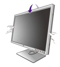
If your monitor is an edge-to-edge monitor, handle it with care. Avoid finger pressure on the screen surface. Adjust the screen angle by placing your hands on the top and on the bottom of the monitor as illustrated. Excessive force on the display is prohibited.
