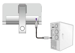
Connect USB devices via other USB ports (downstream) on the monitor. These downstream USB ports transmit data between connected USB devices and the upstream port.
