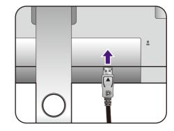
After the monitor and the computer are powered on, if the image is not displayed, disconnect the DP cable. Connect the monitor to any video source other than DP first. Go to **System** and **DisplayPort** on the OSD menu of the monitor and change the setting from 1.4 to 1.1. Once the setting is done, unplug the current video cable and re-connect the DP cable. To go to the OSD menu, see Basic menu operation on page 45.
