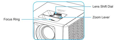
**Note:** The projector will focus at a distance of 1.3m to 9.4m.
