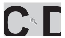
Using the "SET/POINT ZOOM" button on the remote control enlarges part of the screen image. Press the CH+/- button to zoom in or out. The image can be expanded up to 10 times.
