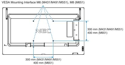
Mounting accessories can be attached with the monitor in the face down position. To avoid scratching the LCD panel, always place a soft cloth, such as a blanket that is larger than the monitor's screen area, on the table before laying the monitor face down. Make sure there is nothing on the table that can damage the monitor.
