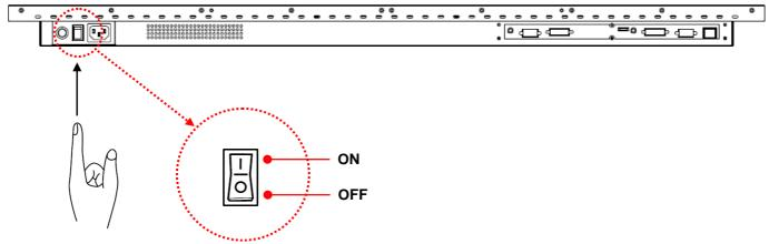
**NOTE:** the remote control only works when the main switch is in the ON position.
