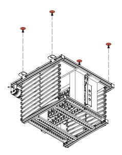
After having fixed the lift to the ceiling, please remove the polystyrene cubes from the lift structure.
