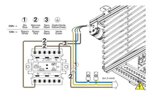
4.5.5 Any operation that will involve electrical components has to be carried out by qualified personnel only, always following the procedure here under:
