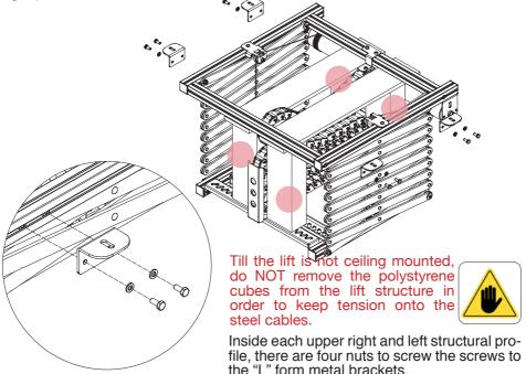
The drawing below indicates the recommended position where to mount the "L" form metal brackets. In this installation manual, we suppose an installation to a flat and horizontal ceiling made of concrete.
