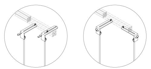
After fixing the threaded bars (fig. 04) and defined the right length, the false ceiling plate can be mounted using two types of screws. The following drawings describe the two types of installation.
