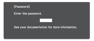
Hold down the [Num] button on the remote control while you enter the password using the numeric buttons.
