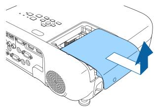
Loosen the screws securing the lamp to the projector. The screws do not come all the way out.
