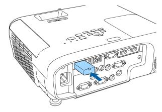
Attach the wireless LAN module cover, and secure it in place with the screw.
