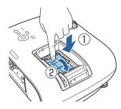
Tighten the two lamp fixing screws.
