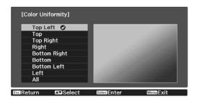
Use the up and down buttons to select the color you want to adjust, and then use the left and right buttons to adjust.
