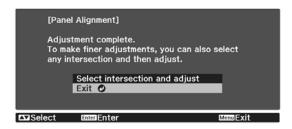
If you feel you still need to make adjustments after correcting all four points, select **Select intersection and adjust** and then continue making adjustments.
