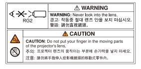
• As with any bright source, do not stare into the beam, RG2 IEC/EN 62471-5:2015.
